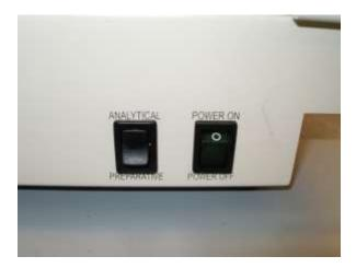
Make sure the first switch is set to **Analytical**. The second switch is used to turn the device on and off. At this point, you can switch on the device and examine your specimen, making sure to stay behind the shield. If you need to work with your sample(eg. To cut your gel), make sure that you are wearing gloves and a lab coat. Turn off the device when you are not looking at the specimen. The lamps on this device quickly burn out if the device is left on for too long.
